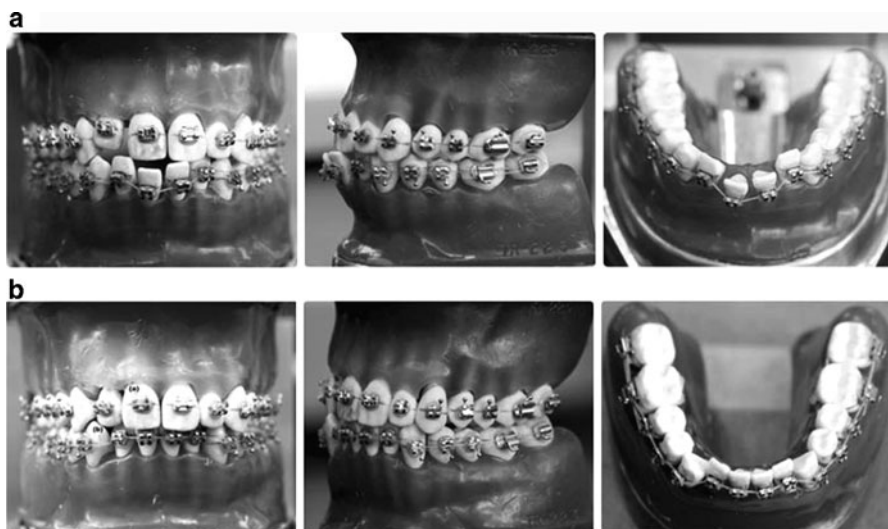
Fig. 9 An SMP archwire was stretched to 50% strain and installed in a dental model with misaligned teeth (a). After heating above T_{\text{trans}} (40°C) to 50°C, the teeth were corrected within 1 h (b). (Reprinted with permission from [68] © 2008, Springer publishing company)
